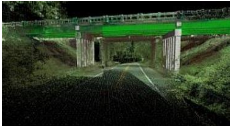
Figure 1: Terrestrial LiDAR technique measuring roadways
